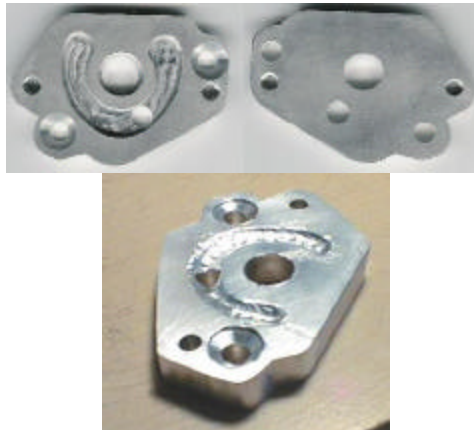
Figure 20: EGR Adapter Plate.
