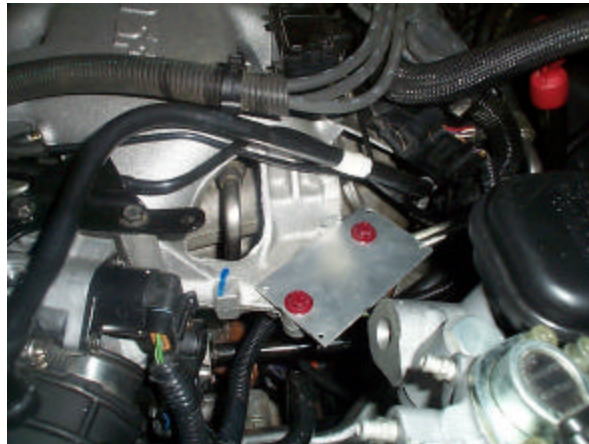
Figure 17: Blocking off the EGR port with a plate.
