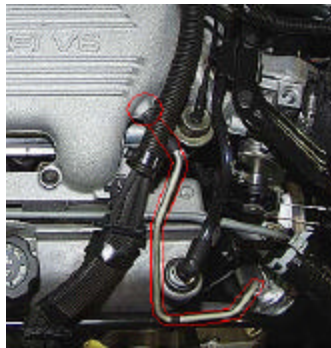
Figure 2: The Modulator Vacuum line on the 3.1.
