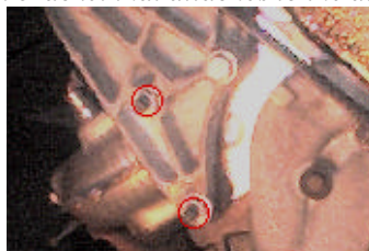
Figure 6: For easier removal/installation, use large pliers on these two bolts.
