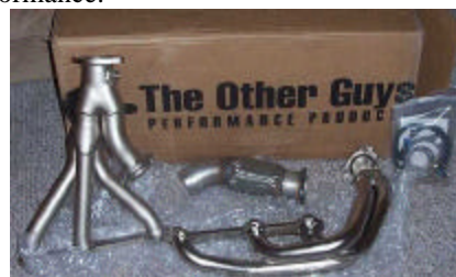
Figure 25: Headers for the 3.4L V6
